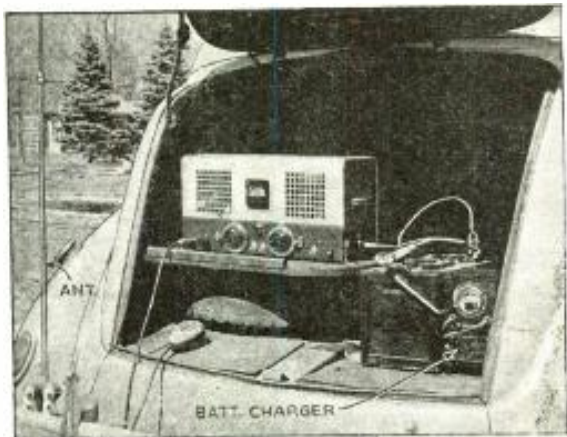
Fig. 2: The complete installation includes transmitter, battery, charger and antenna. Placement of these components will vary with different makes of cars, but battery leads must be kept short.
